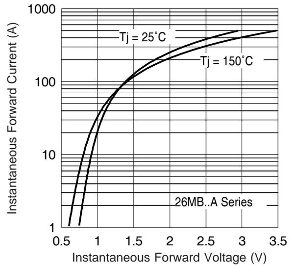
Fig. 2 - Forward Voltage Drop Characteristics
